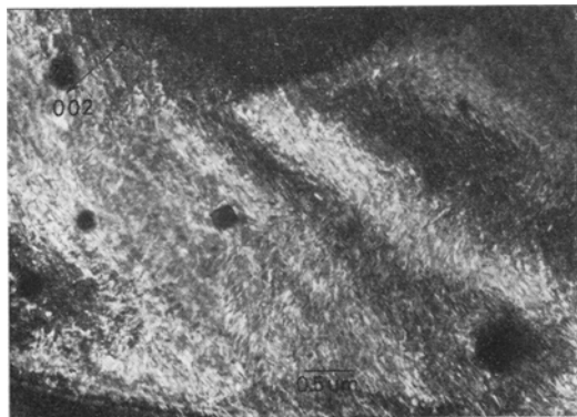
Figure 10 The solution-treated condition aged for 100 h at 315°C, with the intermediate precipitate \gamma' present. (The large regular particles are a Cu-Be-Co compound [18].)
